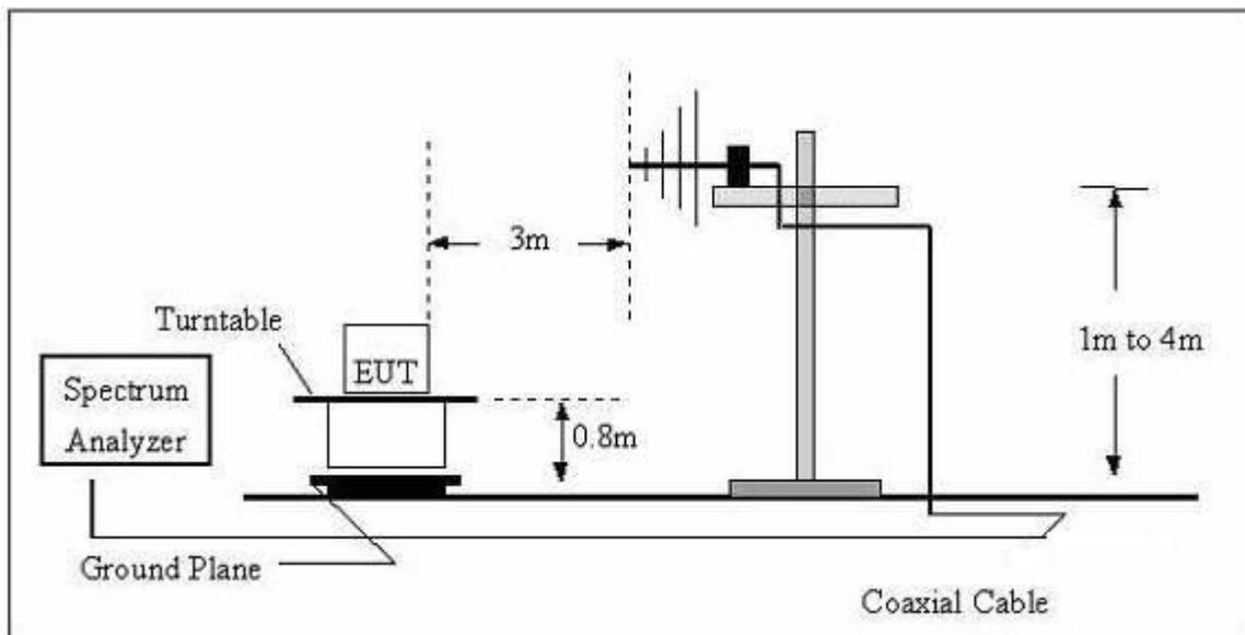
(C) For radiated emissions above 1000MHz
