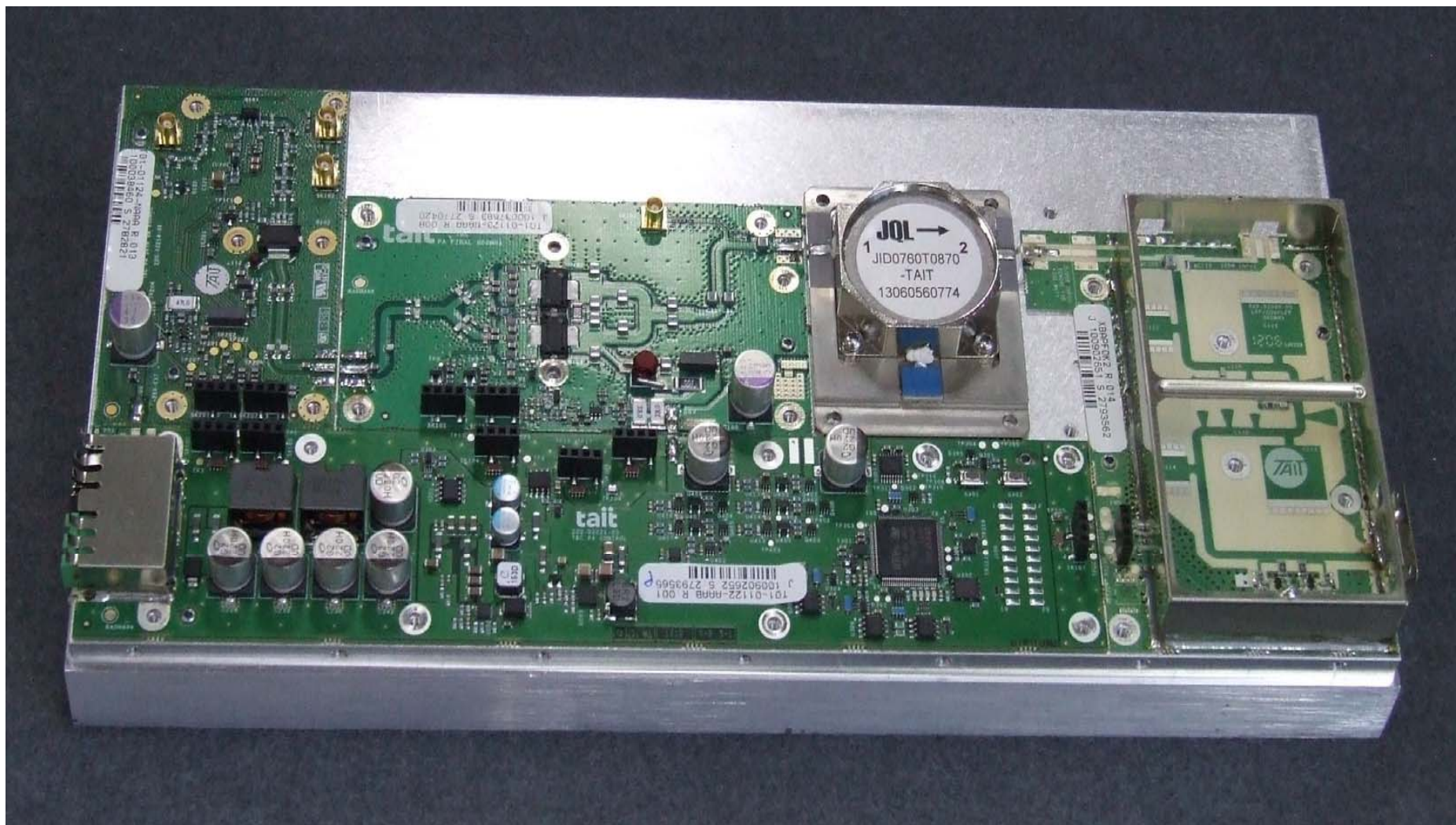
Photograph 02: 50W PA modules – Top. Shields Removed
