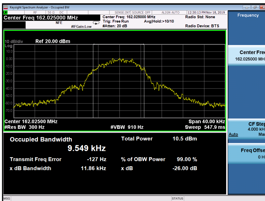
Figure 2 - 162.025 MHz Occupied Bandwidth
