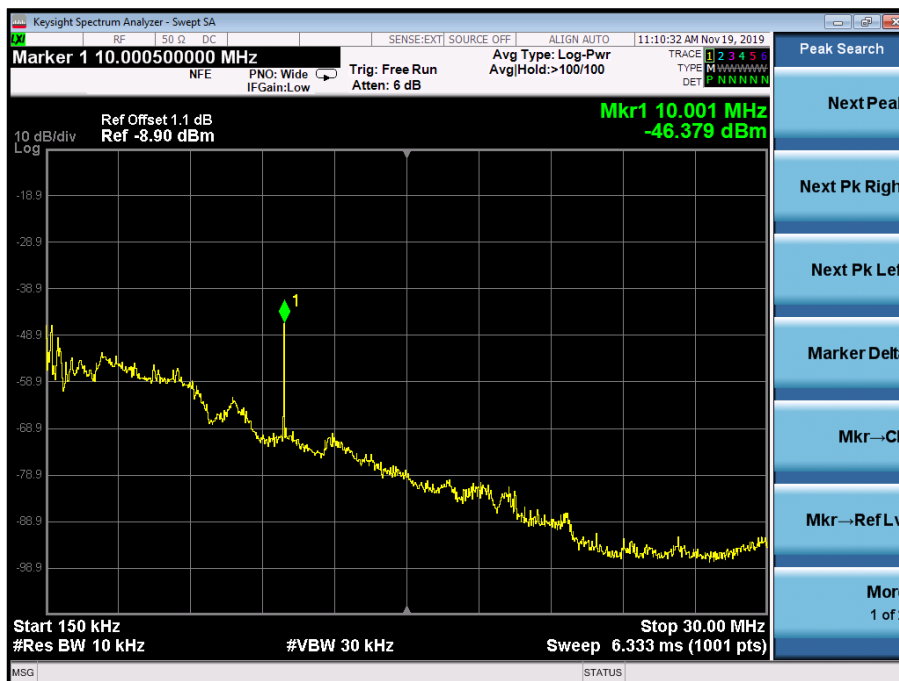
Figure 32 - (156.025 MHz) 150 kHz to 30 MHz
