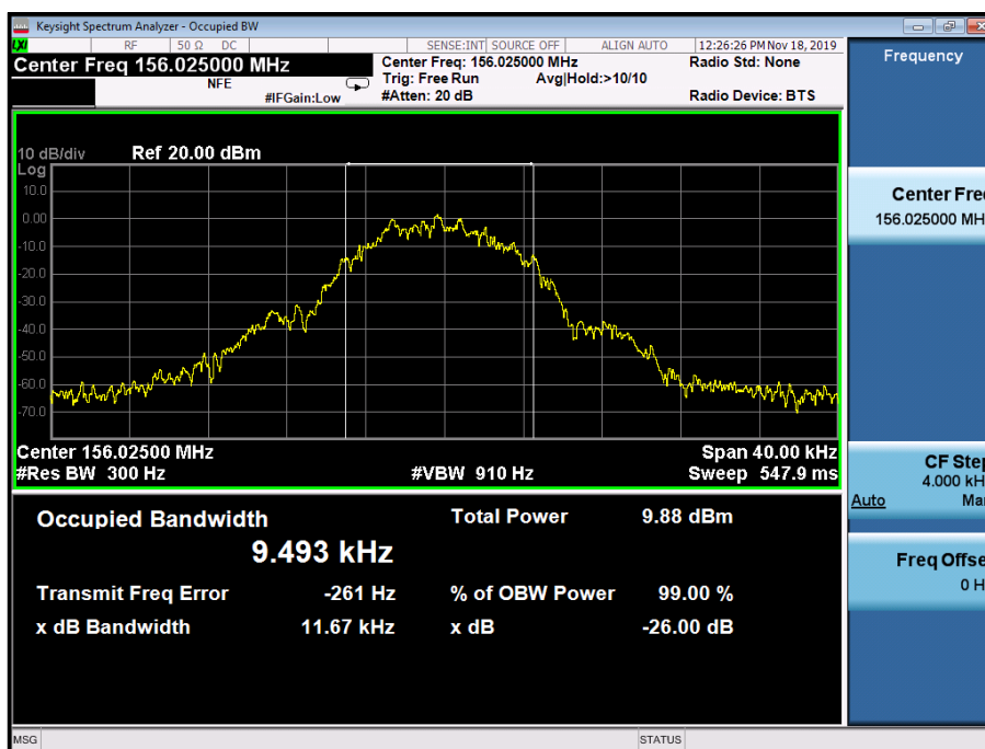
Figure 3 - 156.025 MHz Occupied Bandwidth
