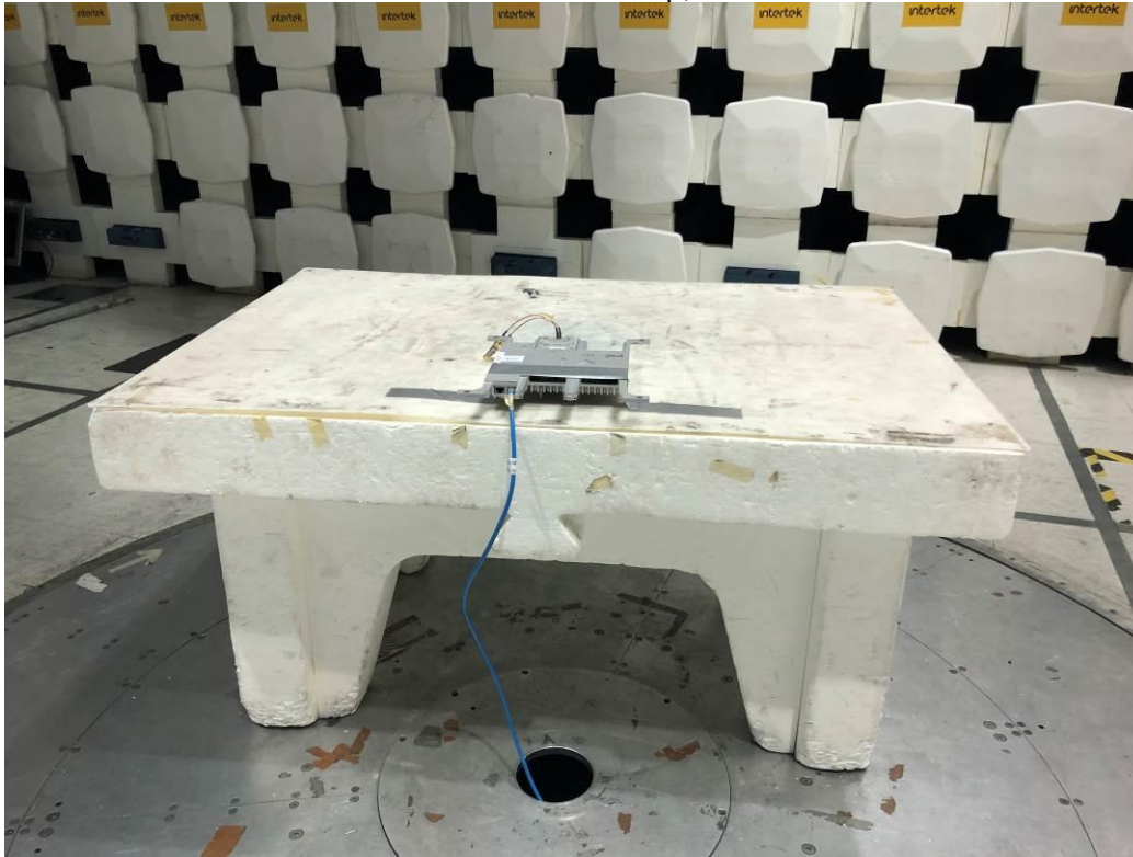
Radiated Emissions Test Setup, 1-12 GHz
