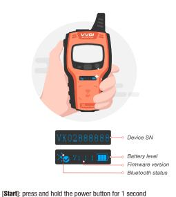
[Shut down]: press and hold the power button for 4 seconds
