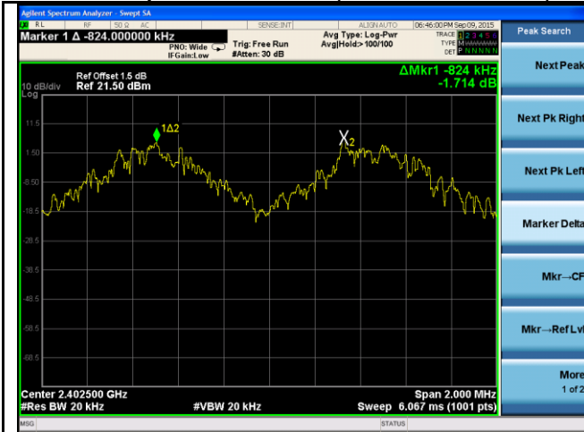
Channel Separation-BDR 2402MHz
