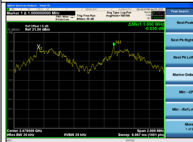
Channel Separation-BDR 2441MHz
