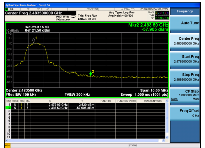
Band Edge-Single-EDR 2480MHz
