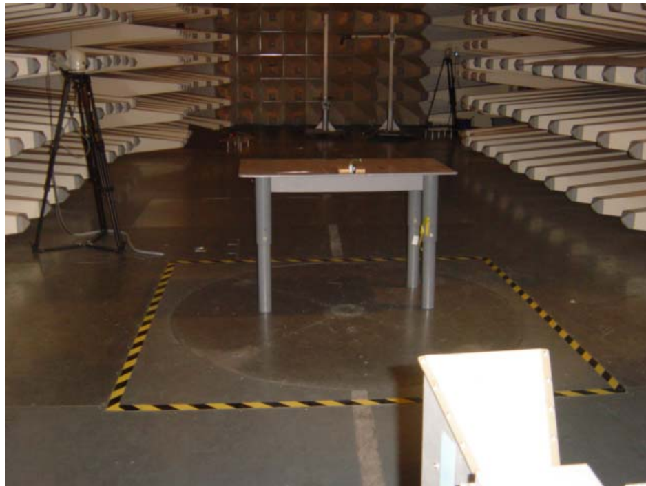
Set-up for Radiation Emission (Transceiver)
