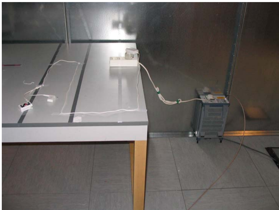
Set-up for Disturbance Voltage on AC mains
