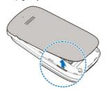
Install the micro-SIM card and the microSDHC card with the cut corner oriented as shown.
