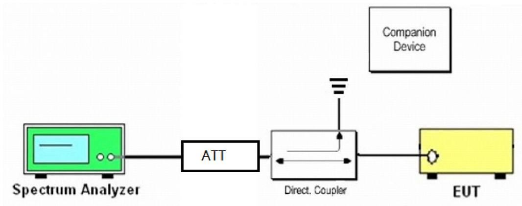
End User Device as UUT, the companion device is certified CBRS (FCC ID: 2AG32PBS31010)
