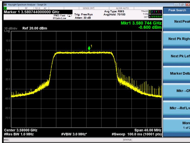
EIRP PSD =  $-0.6 - 4.64 + 6 = 1.96$  dBm/MHz, Antenna gain is  $-4.64$  dBi, the path loss is 6 dB
