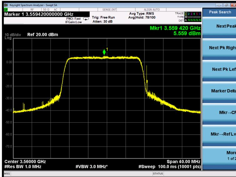
EIRP PSD=5.559-4.64+6=6.919dBm/MHz, Antenna gain is -4.64dBi, the path loss is 6dB
