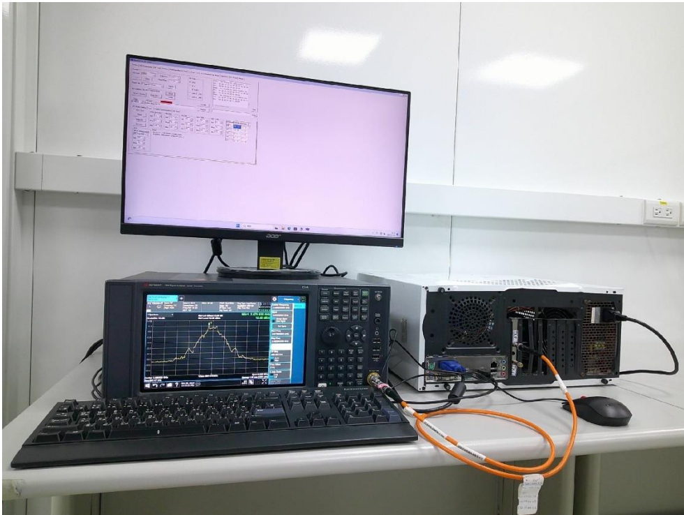
Description: Conducted Emission Test Setup – Wi-Fi
