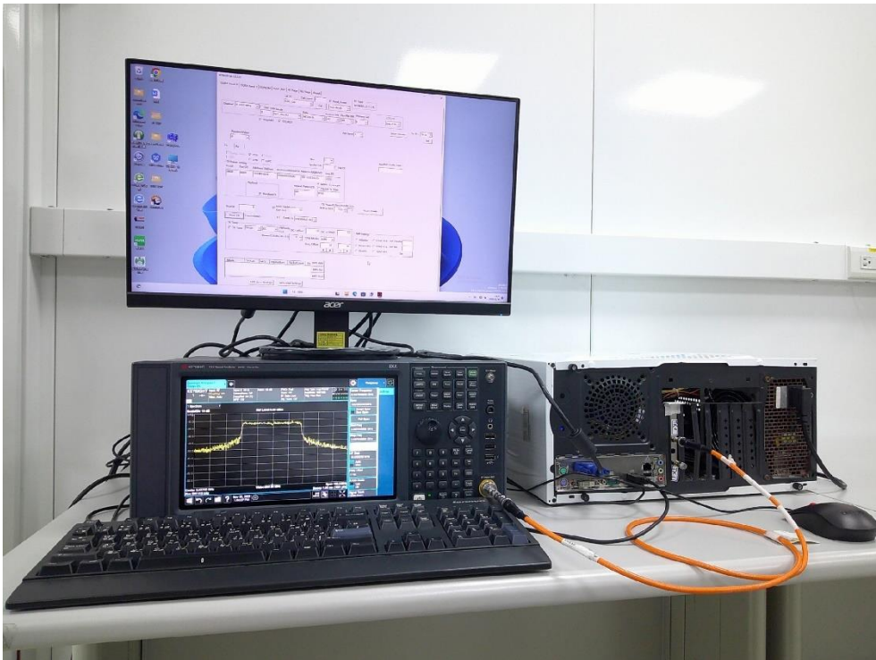
Description: Conducted Emission Test Setup – Wi-Fi
