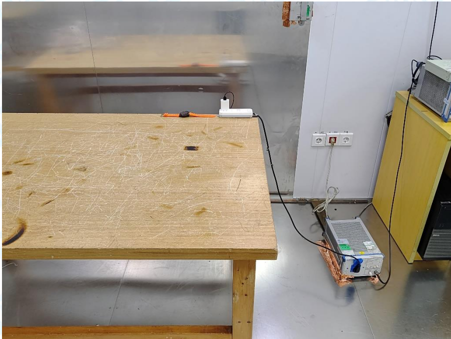
Photo of Setup for Radiated Emission (30MHz~1GHz)
