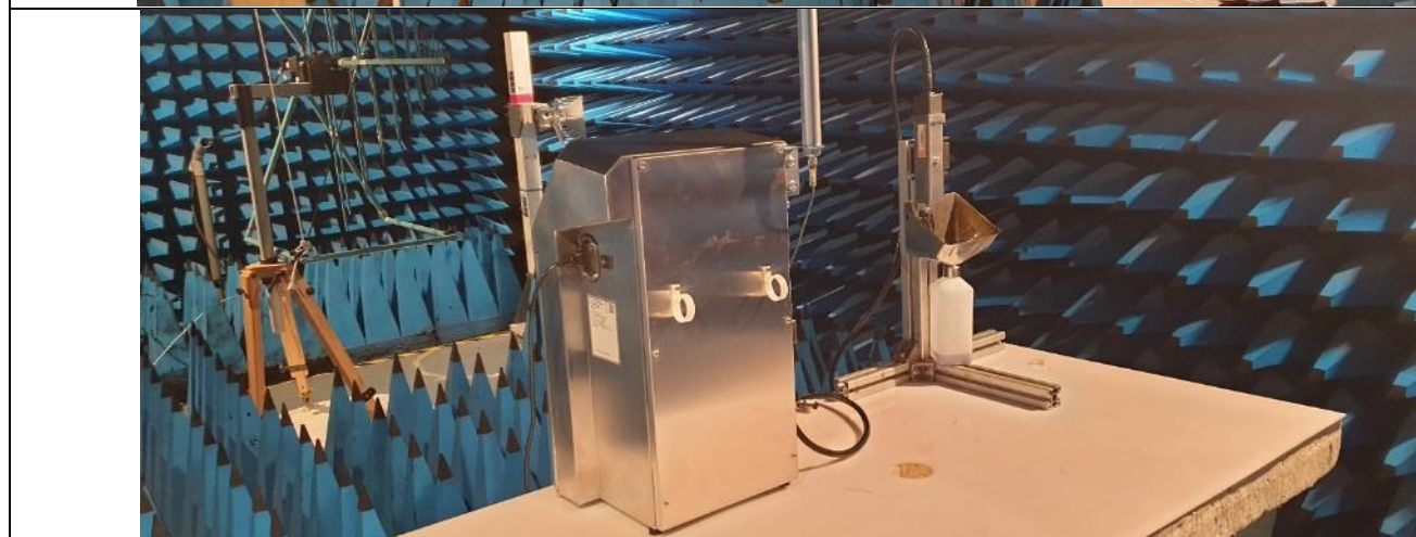
Test setup in anechoic chamber – Frequency <1GHz
