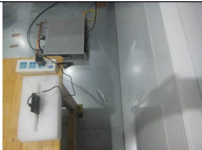
Conducted Emissions Test Setup Side View
