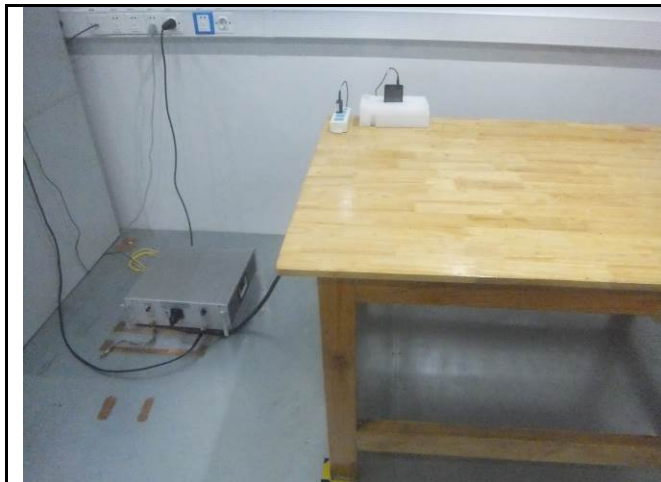
Conducted Emissions Test Setup Front View
