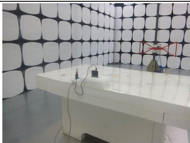
Conducted Emissions Test Setup Front View
