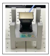
The verification sources apply to system check or verification at specific mmWave frequencies. The sources comprisehorn-antennas and very stable signal generators.
