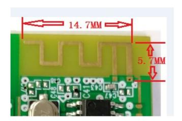
Figure 1 Physical dimension (mm)
