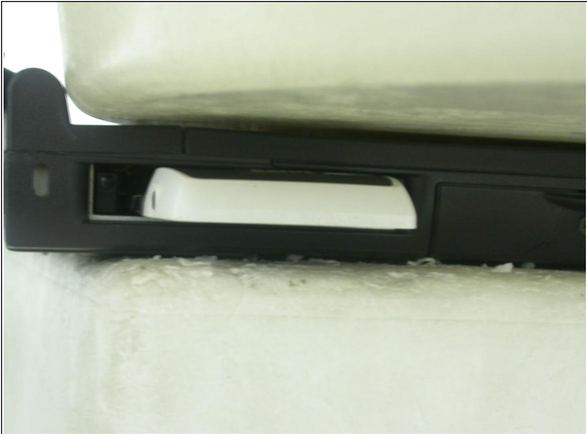
**The EUT to the flat phantom distance is 7mm**
