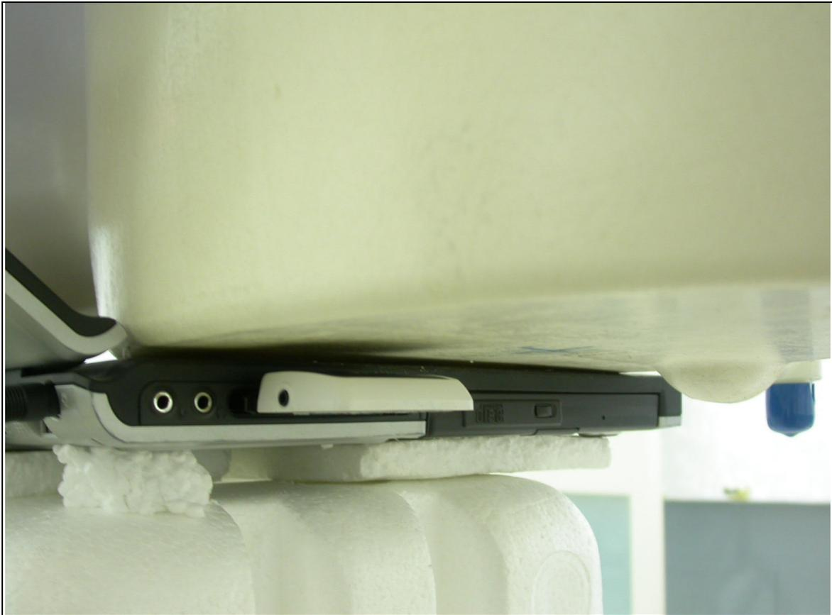
**The EUT to the flat phantom distance is 6mm**
