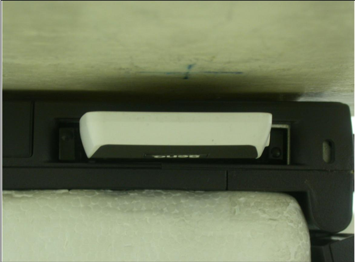
**The EUT to the flat phantom distance is 12mm**
