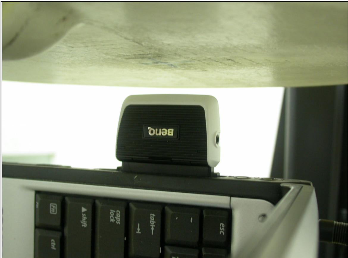
**The EUT to the flat phantom distance is 15mm**
