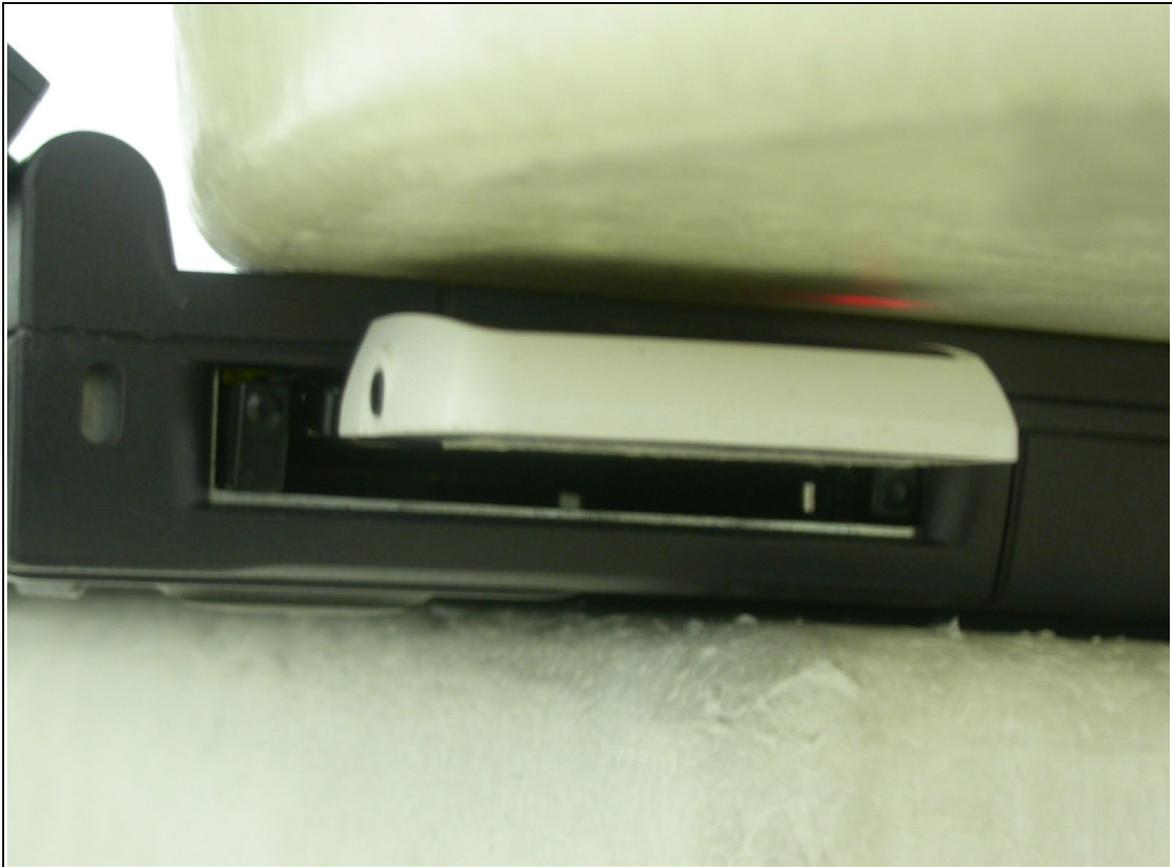
**The EUT to the flat phantom distance is 5mm**
