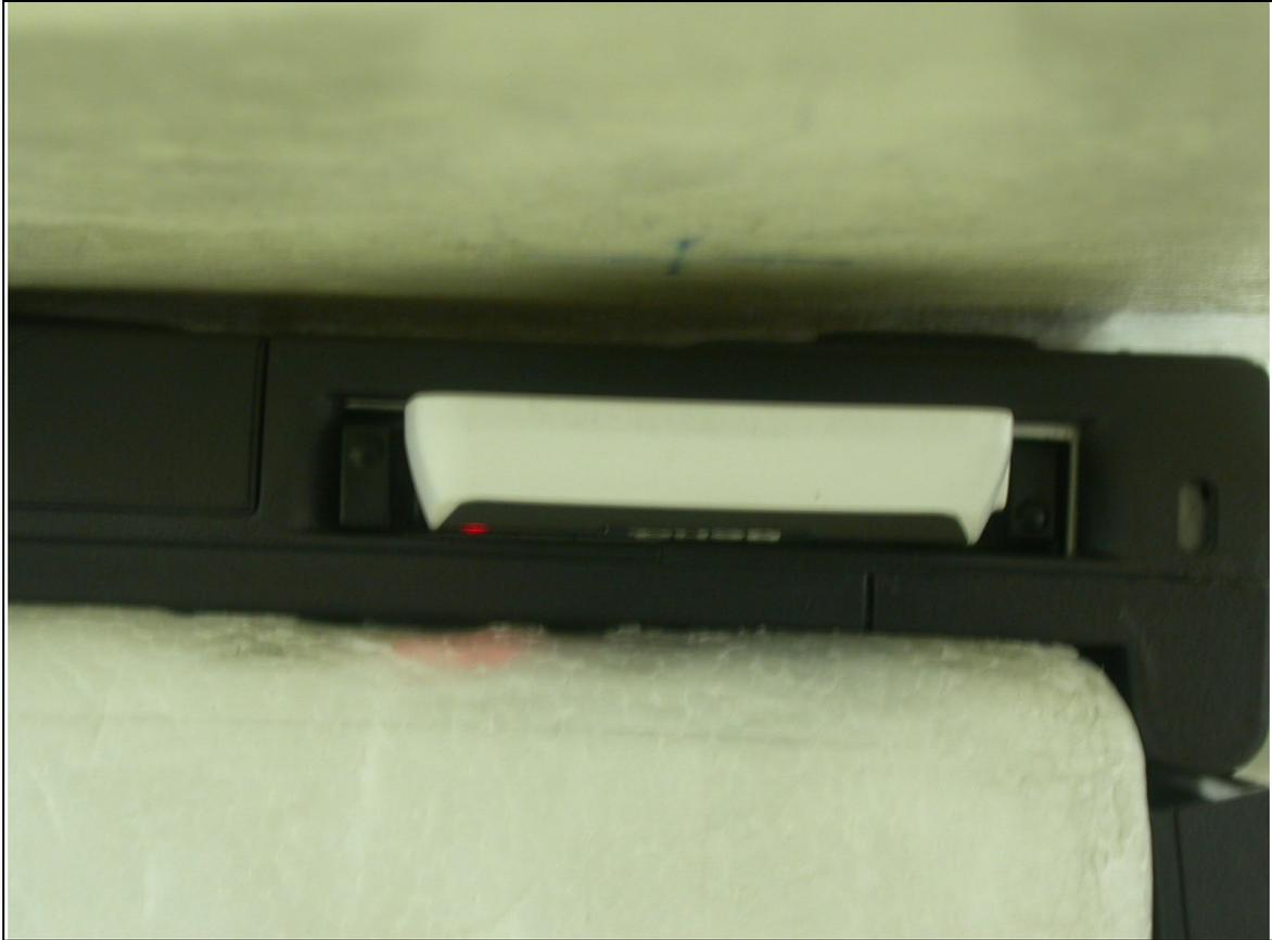
**The EUT to the flat phantom distance is 11mm**
