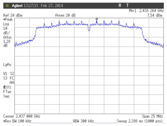
MIMO. Middle Channel: 2437 MHz. Chain A+B. Port A.
