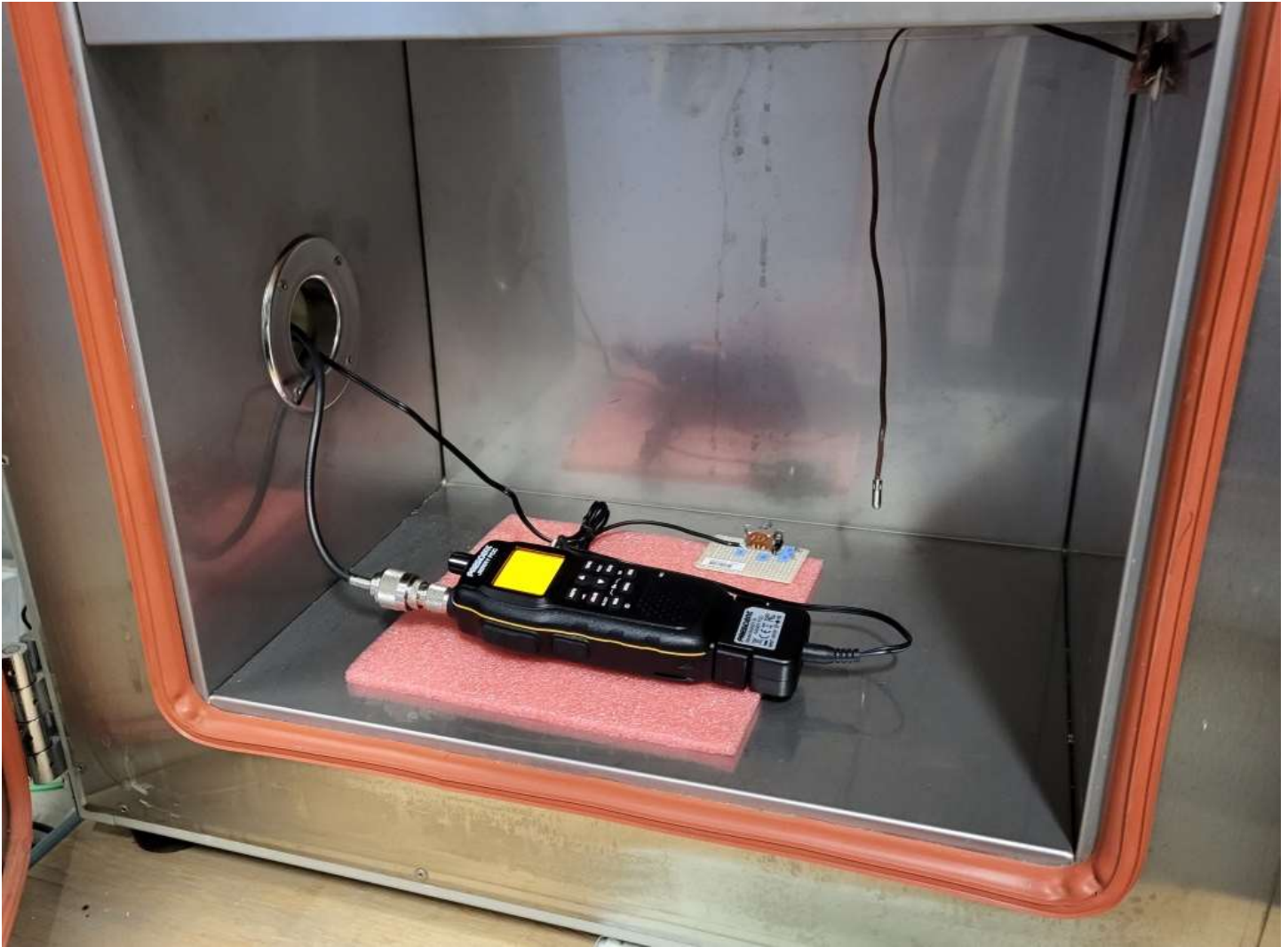
Figure E18.7 – Setup, Frequency Stability
