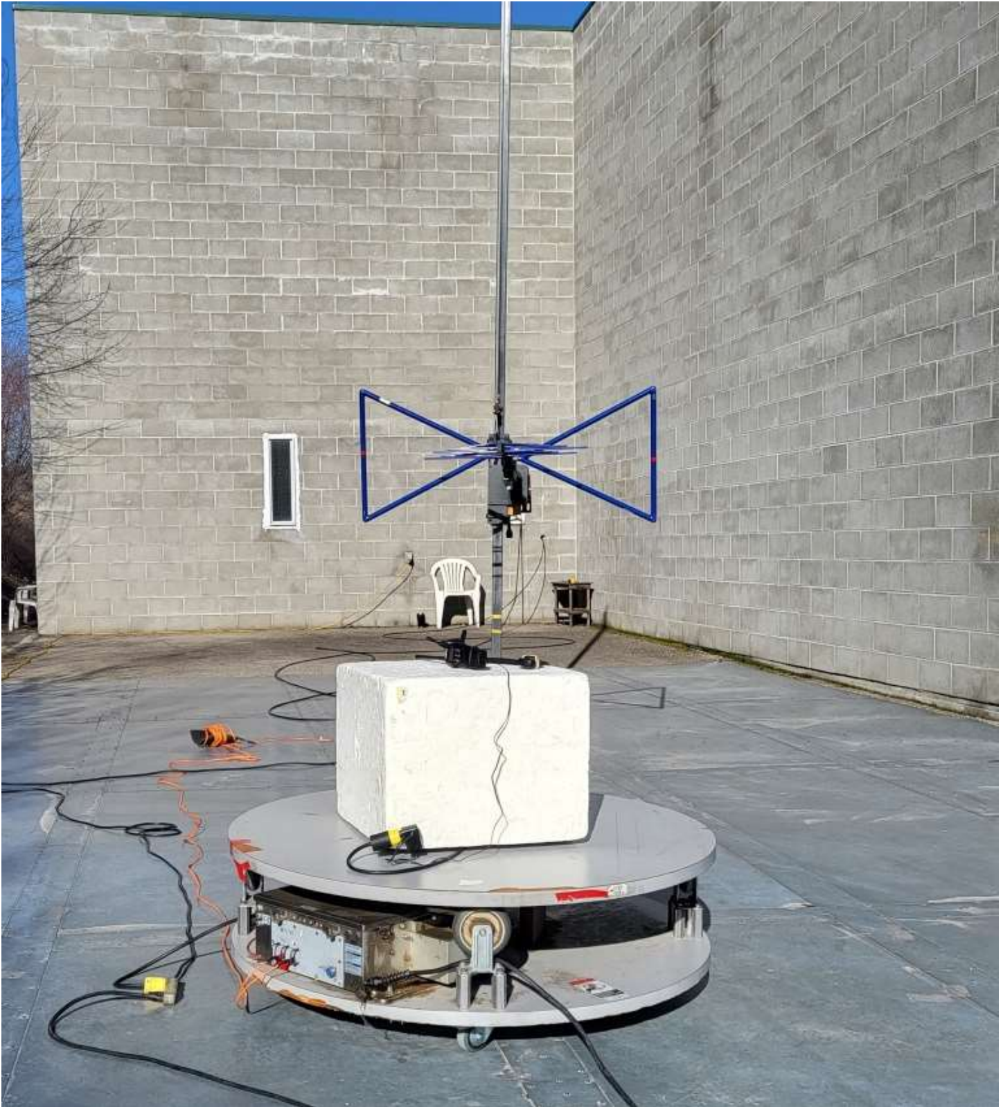
Figure E18.5 – Setup, Radiated Emissions 30 - 1000MHz
