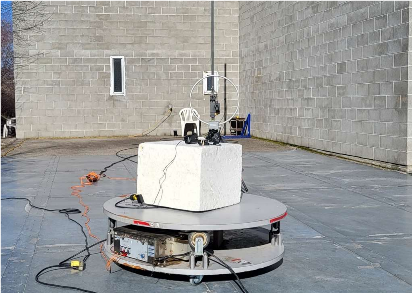
Figure E18.4 – Setup, Radiated Emissions Below 30MHz
