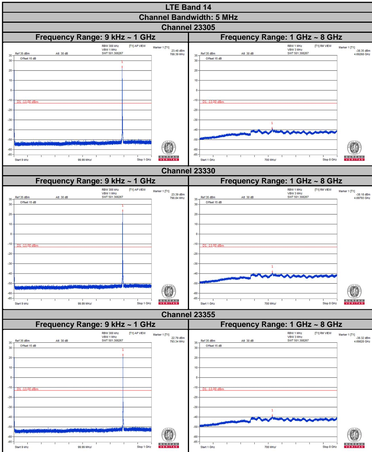
Note: The signal over the limit in 9 kHz is from spectrum analyzer.
