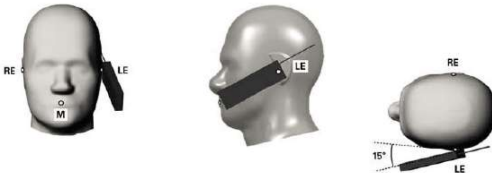
Fig.11.4 Illustration for Tilted Position
