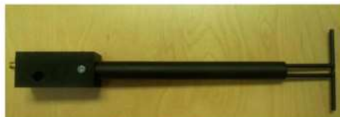
Figure 1 – MVG COMOSAR Validation Dipole
