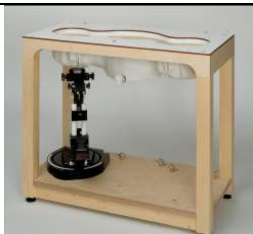
Fig. 8.7 Photo of SAM Twin Phantom
