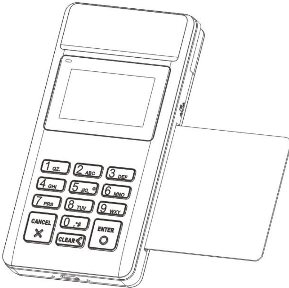
Figure 4. Insert smart card
