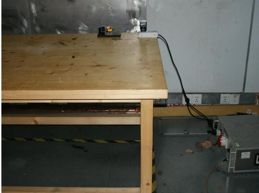
**Photograph 2: Set-up for Radiated Emission, 30MHz - 1GHz**
