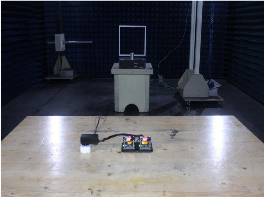
**Photograph 4: Set-up for Radiated Spurious Emission, 30MHz - 1GHz**
