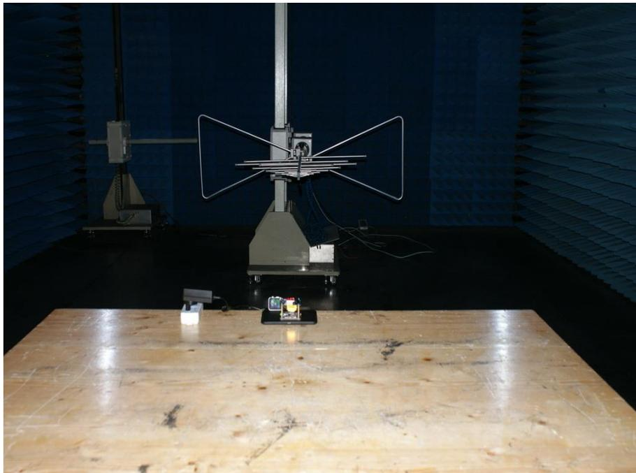
**Photograph 3: Set-up for Radiated Spurious Emission, 9KHz - 30MHz**
