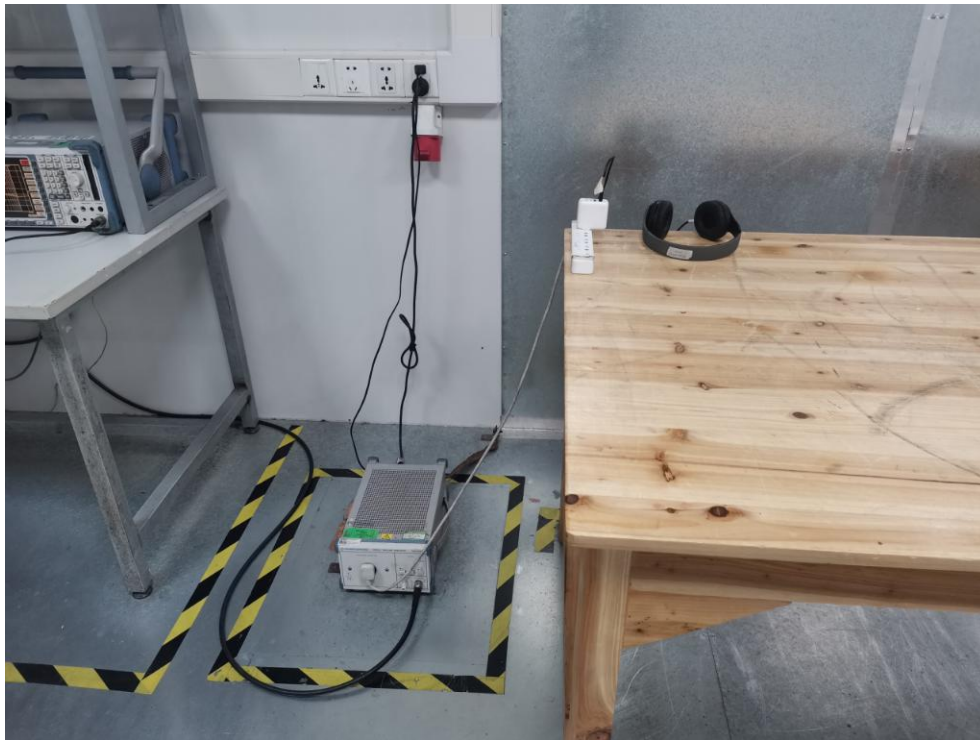
FCC ID: 2AJQ7LOGO Photo of Conducted Emission Measurement
