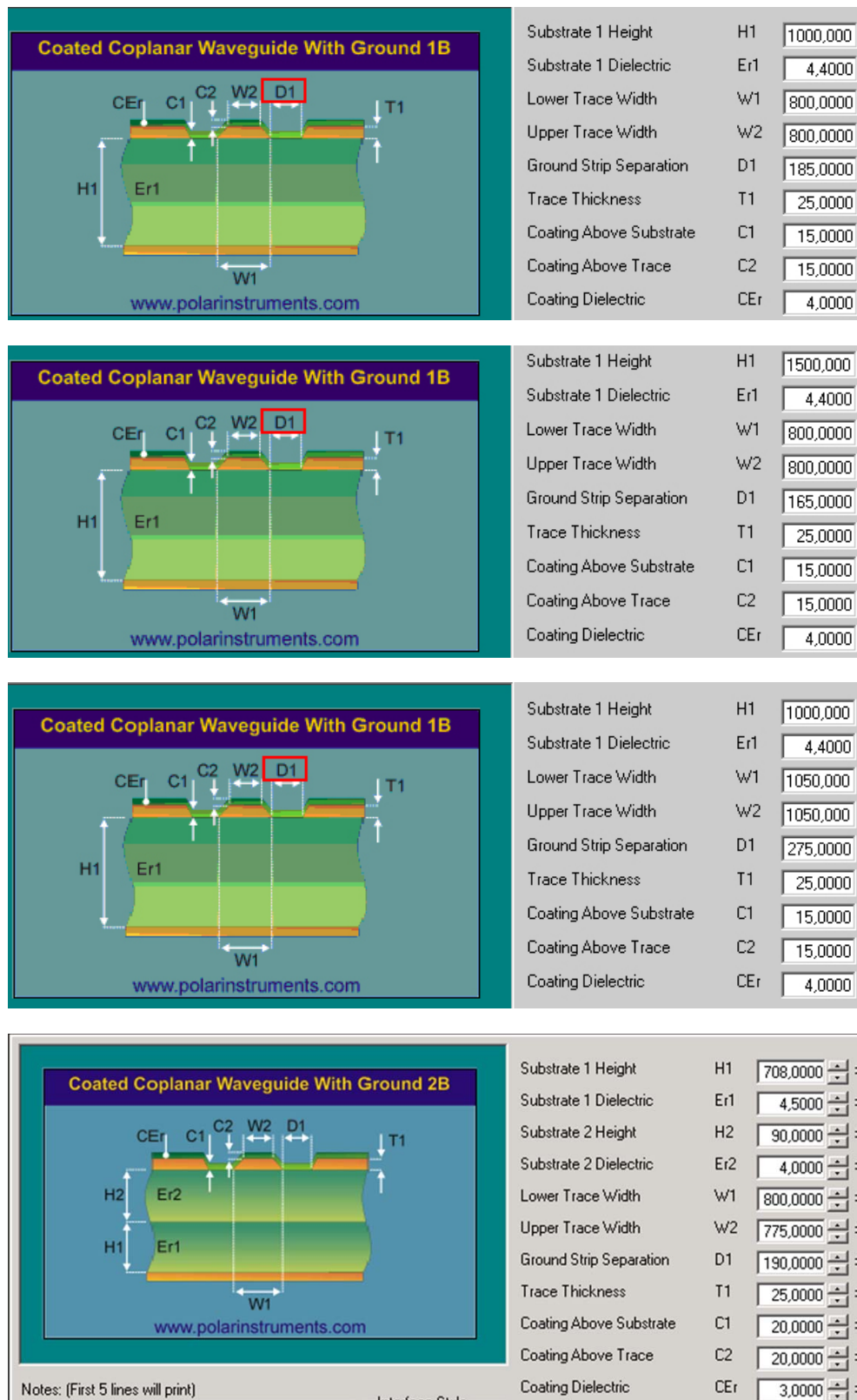
Figure 6: Micro-Stripline line arrangement samples
