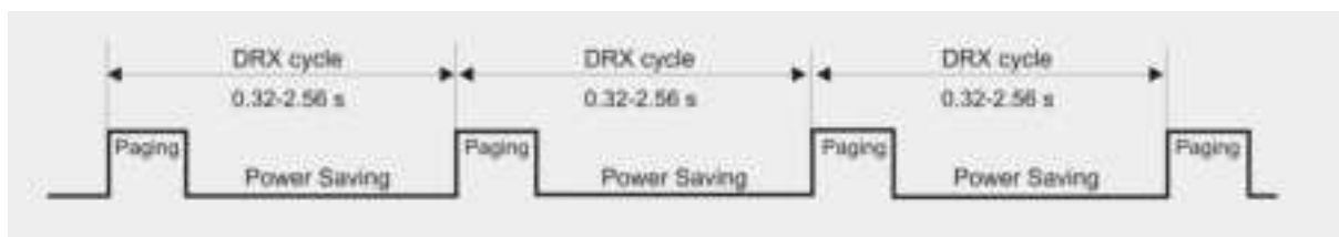
Figure 11: Power saving and paging in LTE networks
