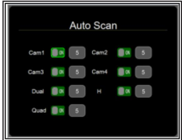
Auto scan duration range is 5-60 seconds. The duration indicates how long a camera view will be shown when the monitor is set to auto scan, before cycling to the next camera view. Each camera view can be turned on or off to be included or removed from the auto scan rotation.
