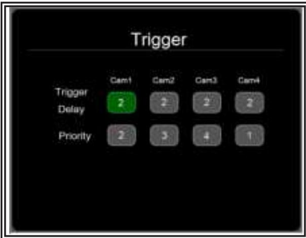
Trigger Delay: setting range is 1-60 seconds. The trigger delay indicates how long it will take after the trigger wire is disconnected, before the monitor goes back to the original view.
