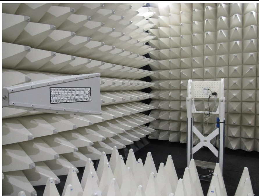
Radiated test setup above 1 GHz for TX mode
