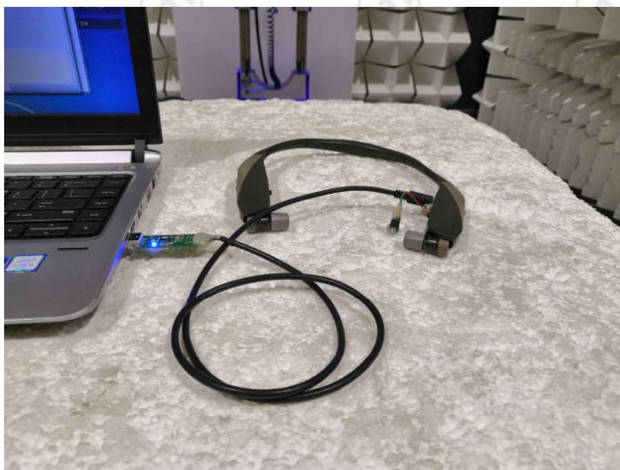
Radiated spurious emission Test Setup for Close-up
