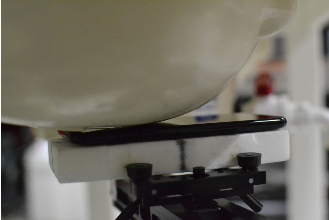
SAR Test Setup Photo 1 – Right Cheek
