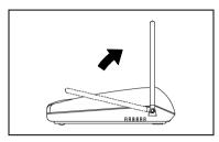
For the best communications place antenna in full upright position before using your FRS Base station.
