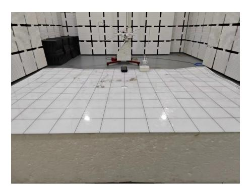
Set-up for Radiated Emission (RE), Above 1GHz
