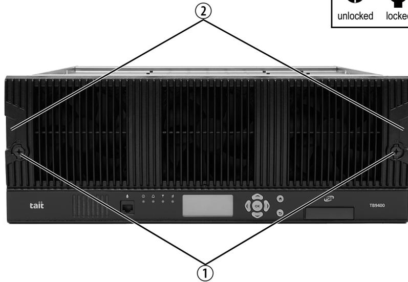
2. Place a finger in the recess ② provided at each end of the front panel and pull the front panel away from the subrack.
