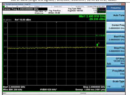
Out-of-band (single test signals) / BRS/EBS / Downlink / 5G NR 20 MHz / Lower
