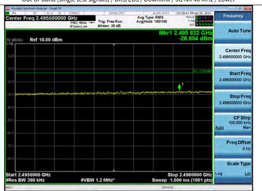
Out-of-band (single test signals) / BRS/EBS / Downlink / 5G NR 40 MHz / Lower
