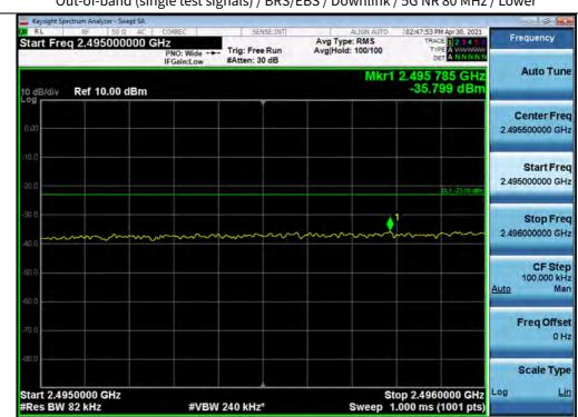
Out-of-band (single test signals) / BRS/EBS / Downlink / 5G NR 80 MHz / Lower
