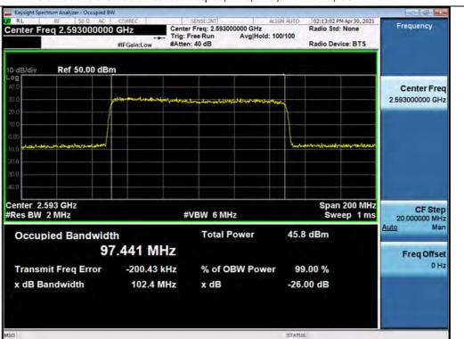
3 dB above the AGC threshold output / BRS/EBS / Downlink / 5G NR 100 MHz
