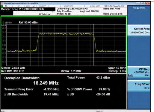
3 dB above the AGC threshold output / BRS/EBS / Downlink / 5G NR 20 MHz
