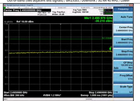
Out-of-band (two adjacent test signals) / BRS/EBS / Downlink / 5G NR 40 MHz / Lower
