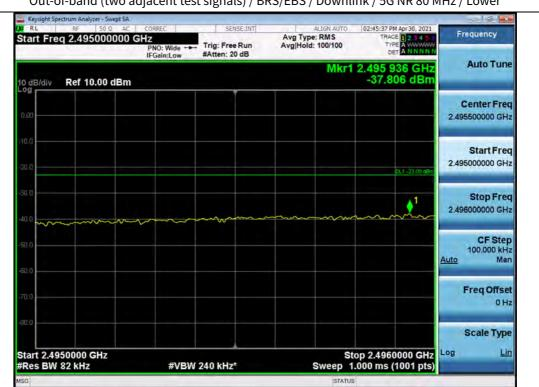
Out-of-band (two adjacent test signals) / BRS/EBS / Downlink / 5G NR 80 MHz / Lower
