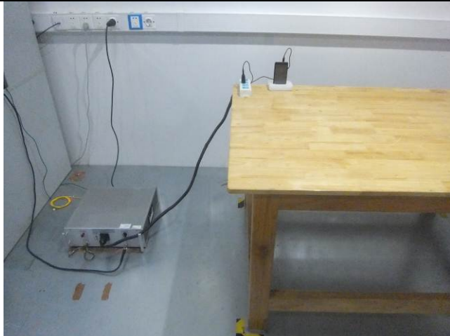
Conducted Emissions Test Setup Front View
