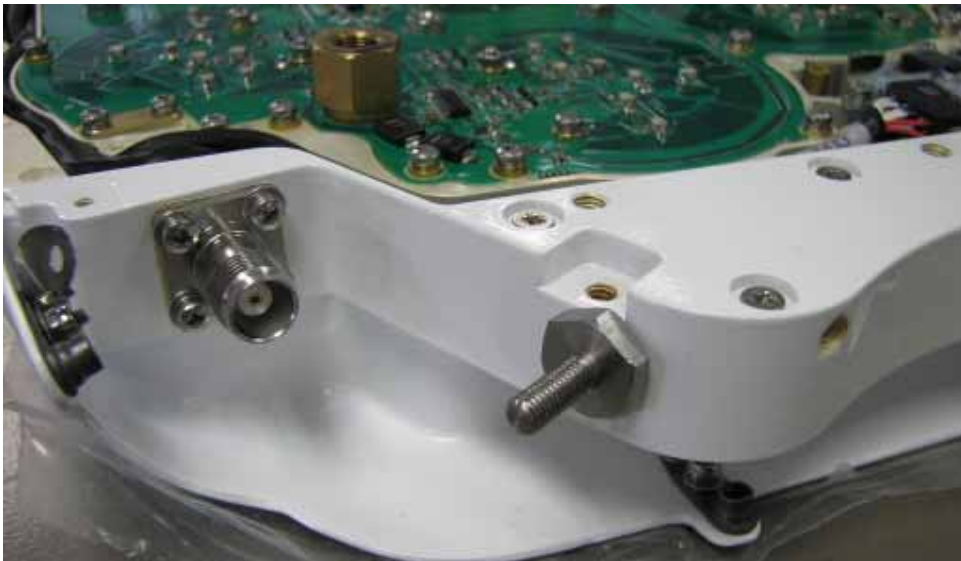
Figure 8: The additional grounding stud on the HGA-7001
