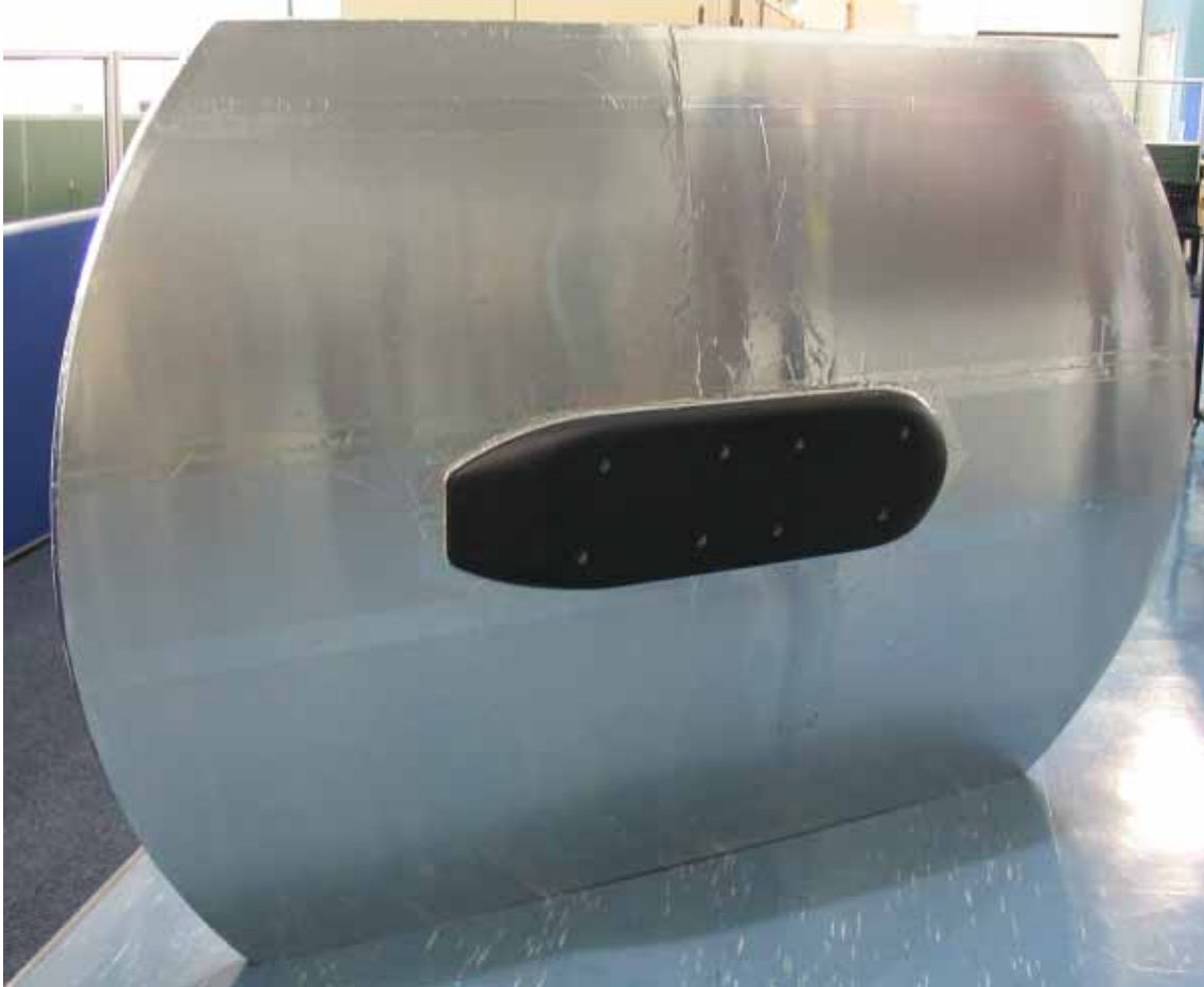
Figure 5: An HGA-7001 on the ARINC 781 ground plane
