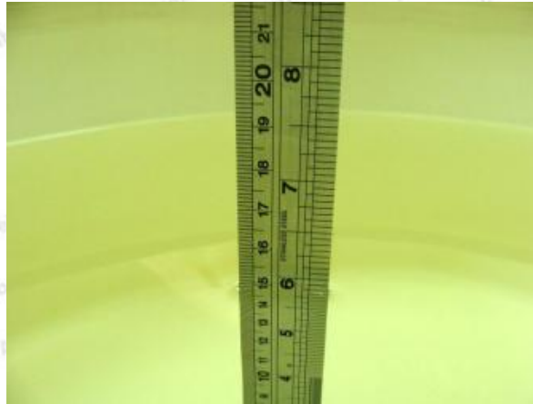
Photo of Liquid Height for Body SAR
