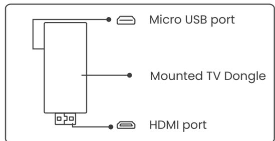
3. Insert the Dongle into its compartment. (Make sure the Dongle is firmly inserted to be recognized.)
