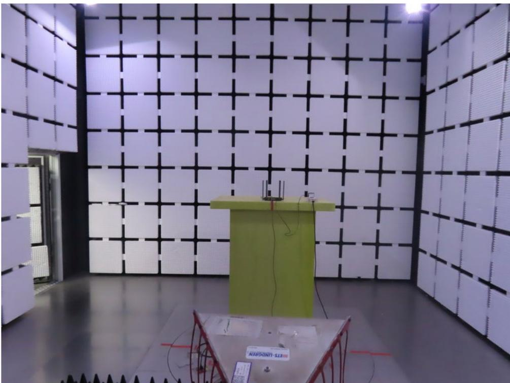
**Radiated Emissions Test Photos****Above 18 GHz**
