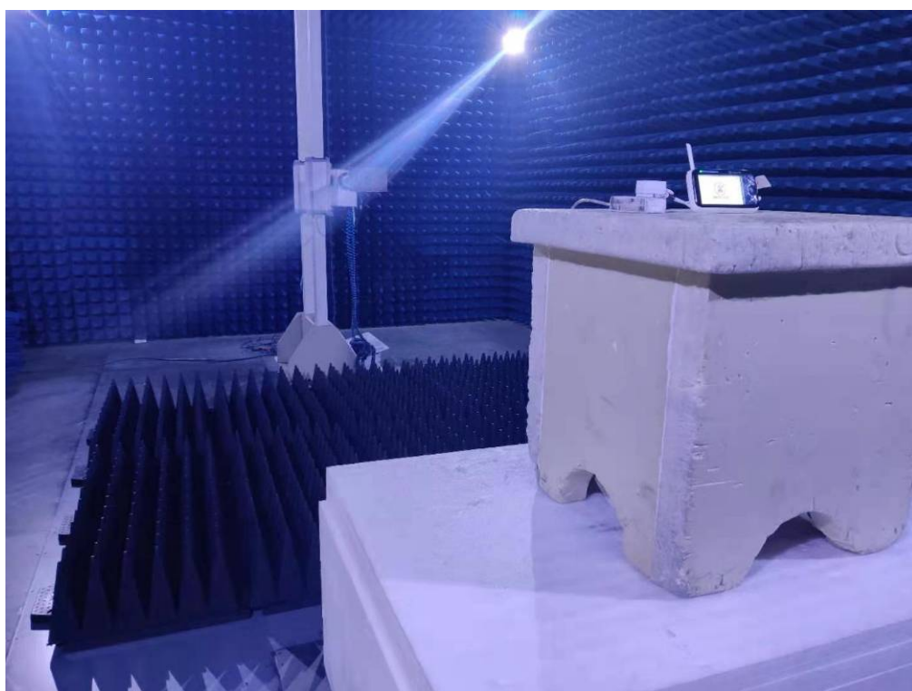
Photo of Radiated Emission Measurement (Above 1G)
