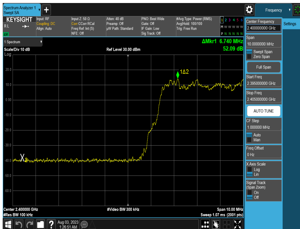
Plot 7-13. Band Edge Plot (Bluetooth with Hopping Enabled, 8DPSK, ePA)
