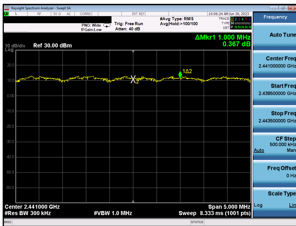
Plot 7-16. Channel Spacing Plot (Bluetooth, 8DPSK, ePA)
