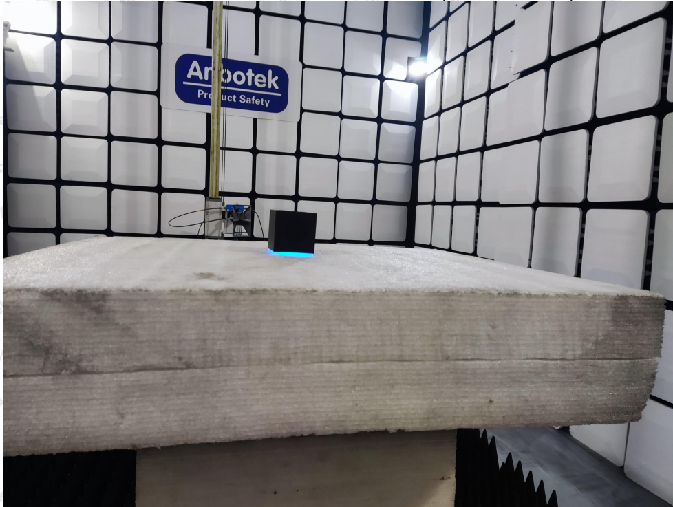
Photo of Radiation Emission Test (above 1GHz)
