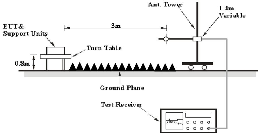
The radiated emission tests were performed in the 3 meters test site, using the setup accordance with the ANSI C63.4-2009. The specification used was the FCC 15.209, and FCC 15.247 limits.
