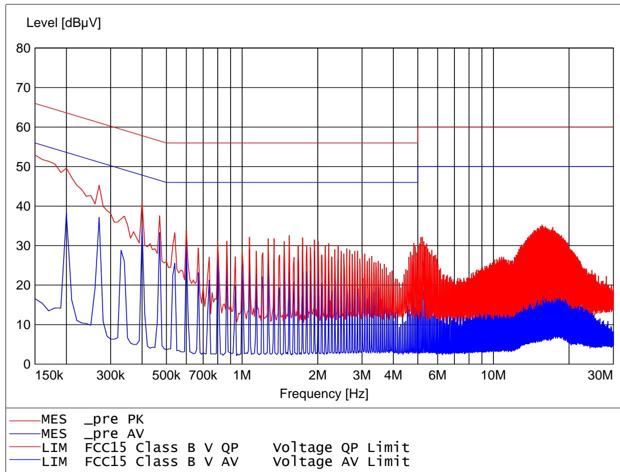
**EMI voltage test in the ac-mains according to FCC Part 15**
