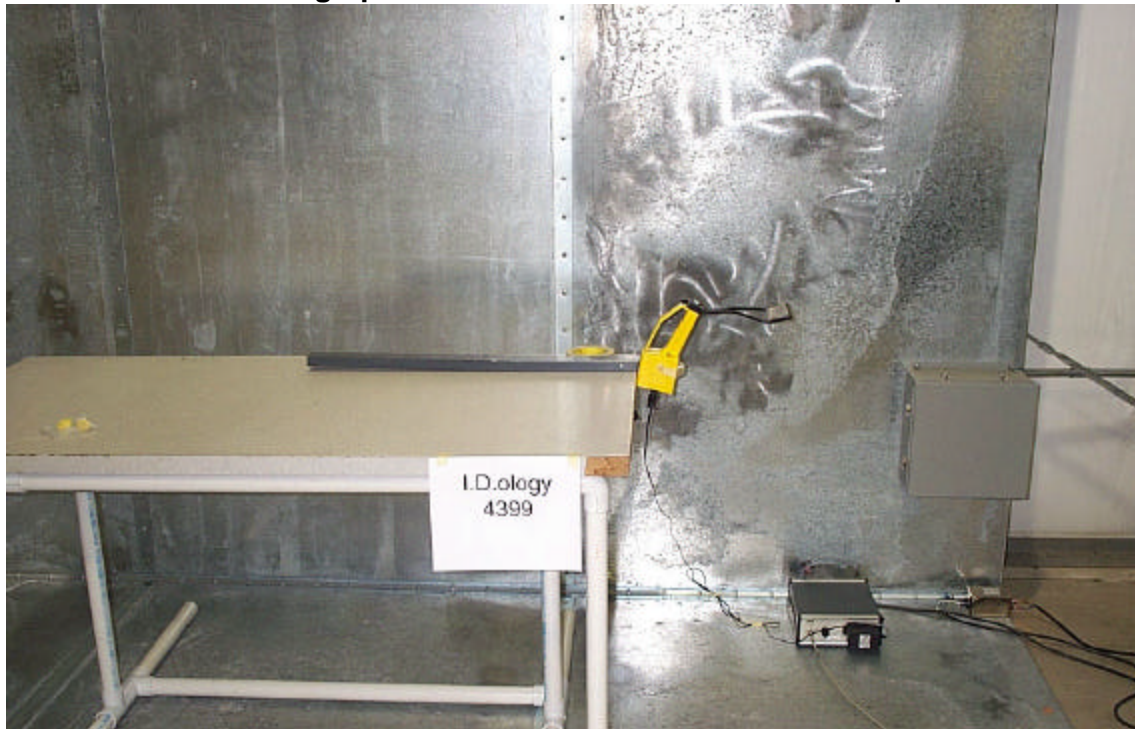
Photograph of Conducted Emissions Test Setup
