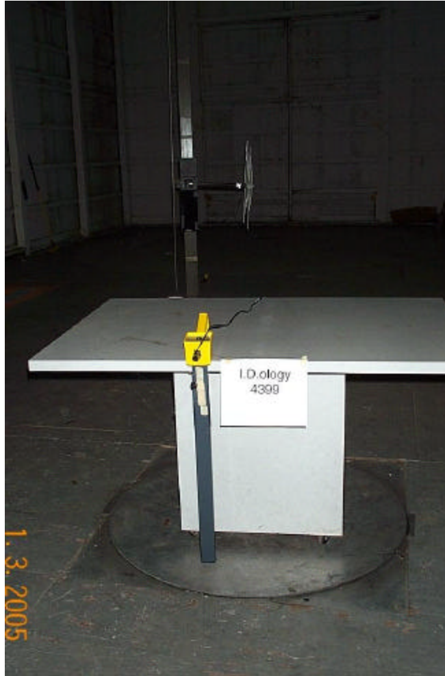
Photograph of Radiated Emissions Test Setup
