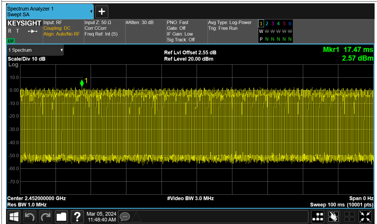
Duty Cycle NVNT n40 2452MHz Sum
