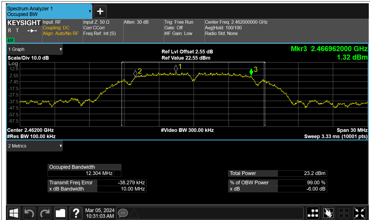
-6dB Bandwidth NVNT b 2412MHz Ant2
