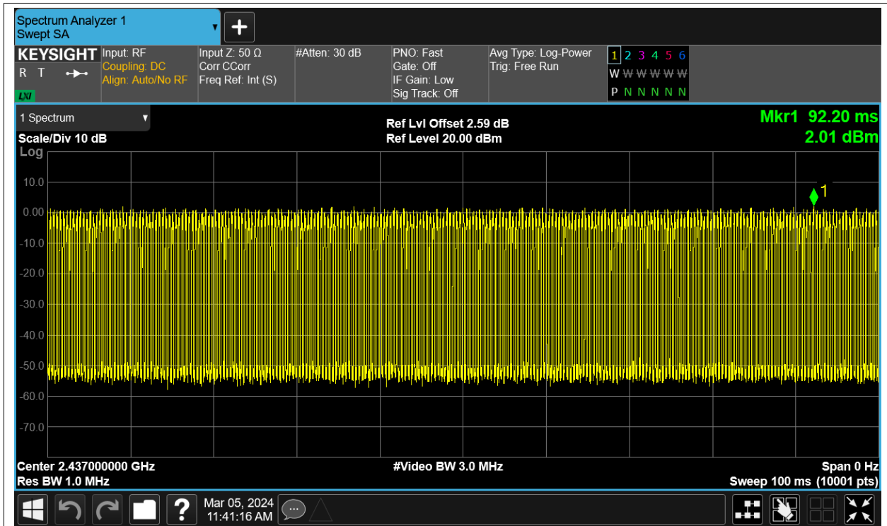
Duty Cycle NVNT n40 2452MHz Sum
