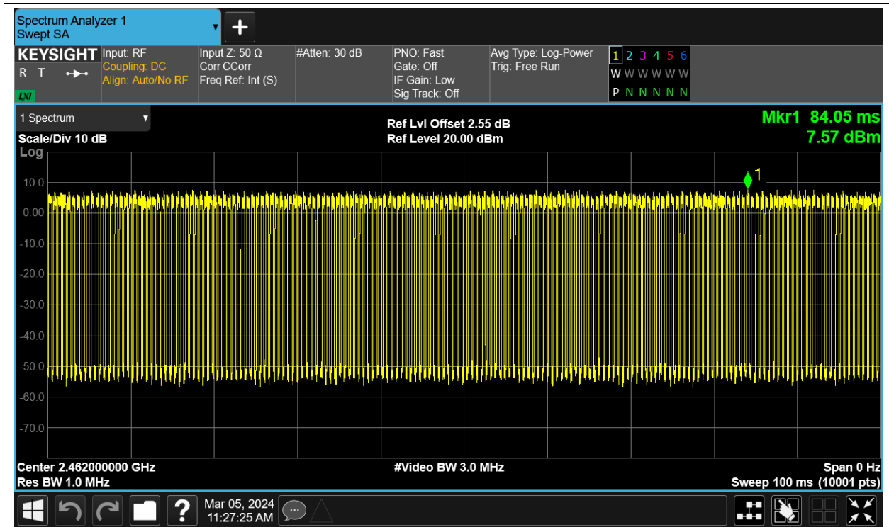
Duty Cycle NVNT n40 2422MHz Sum
