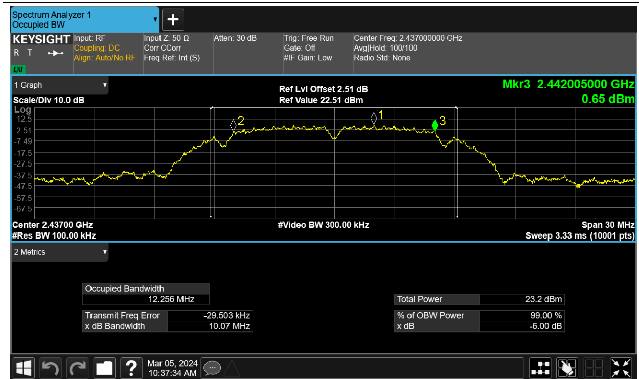
-6dB Bandwidth NVNT b 2462MHz Ant2
