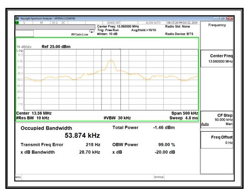
Note: Because the measured signal is CW or CW-like, adjusting the RBW per C63.10 would not be practical since the measured bandwidth will always follow the RBW.
