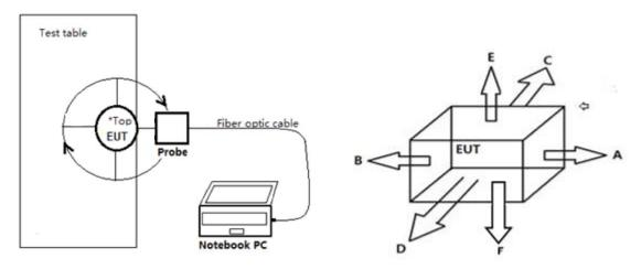
The test distance between the edge of the EUT and the probe center is 20cm
