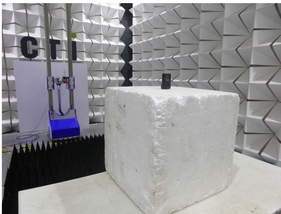
Radiated spurious emission Test Setup-2(Above 1GHz)
