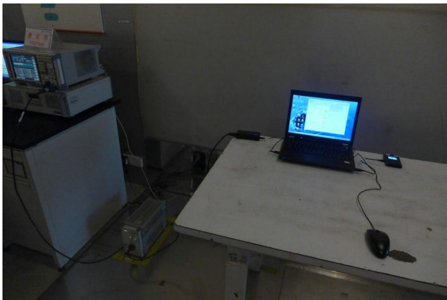
Conducted Emissions Test Setup
