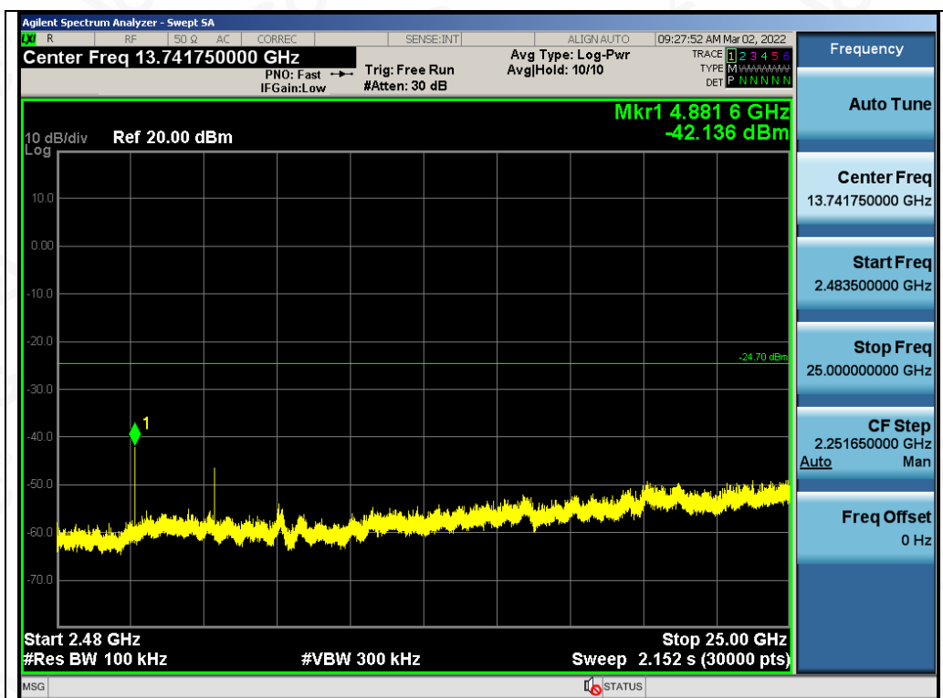
Test_Graph_EDR_ANT1_2441_2Mbps_Higher Band Emissions
