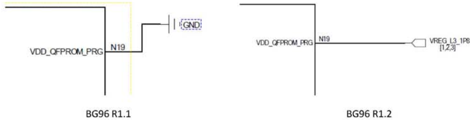
Figure 1: Schematic Designs of BG96 R1.1 and R1.2
